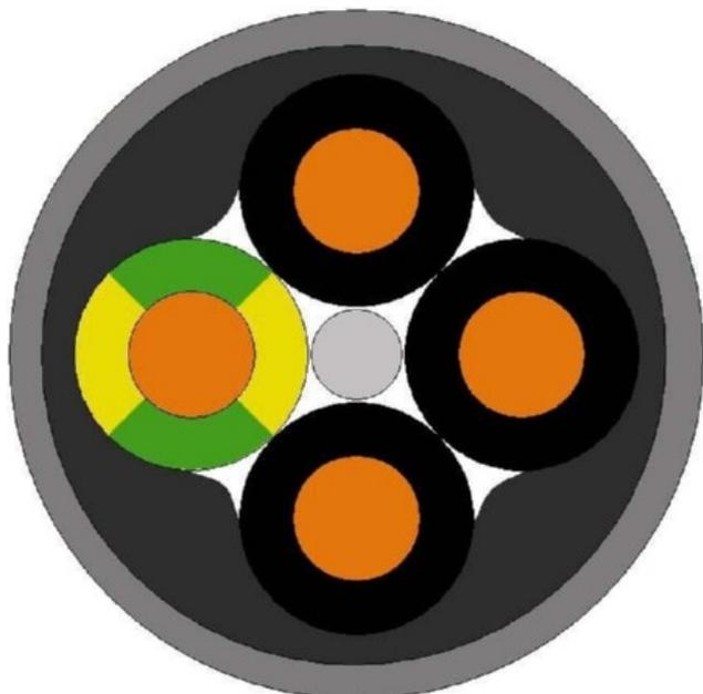
**OELFLEX SMART 108 5G1.5 - Cable d'alimentation <1kV, installation fixe 13050099 R100**
