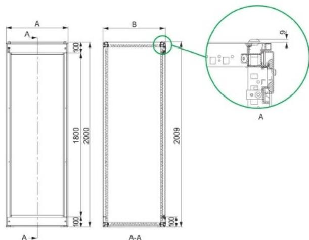
**Armoire de commande 2000x800x600mm IP55
